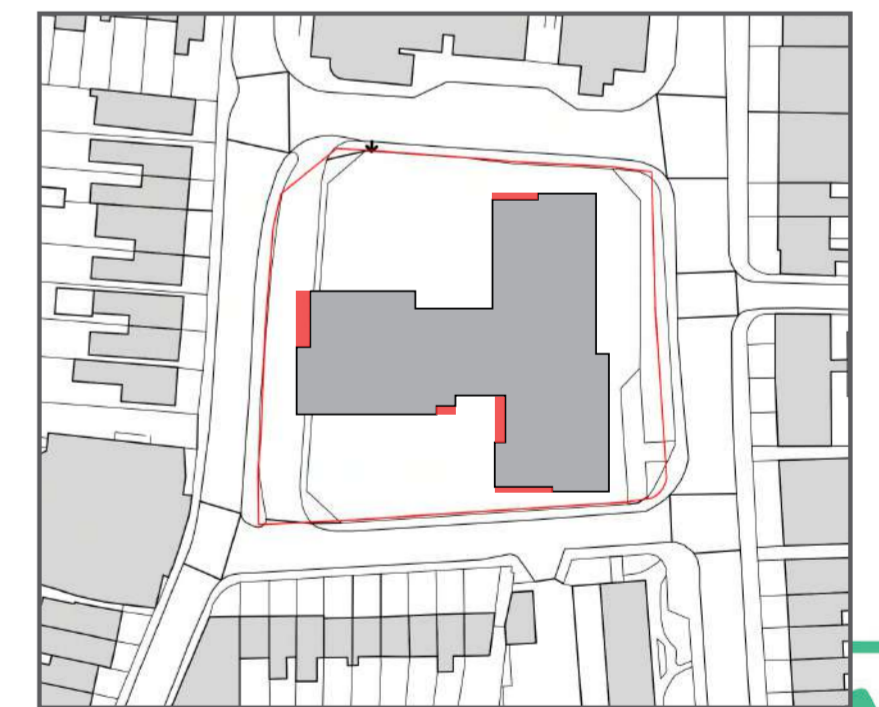
Secondary articulation added through projections / steps in the building line and breaks at roof level to break the form down into a comparable scale to the surrounding context.
